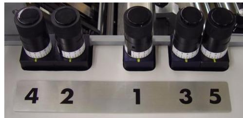
Exclusive, fast and accurate setup of folding roller pressure using the BaumQuick paperless gapsets
