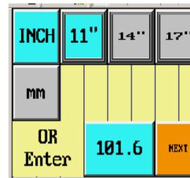
The lengths of standard paper sizes are shown and if you are going to fold one of these simply touch the appropriate one and it will turn blue indicating this is the size you have selected. On this screen you also have the option of selecting either inch or metric measurements.
