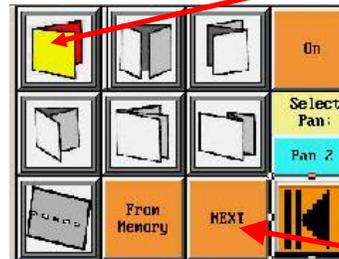
**(B)** When you have selected the type fold, touch NEXT on the control panel. This will bring up the length screen where you will enter in the length of the sheet being folded.
